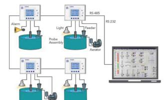
**Example of four monitors individually** monitoring and controlling four tanks on the same network.
